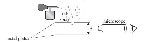
Negatively charged oil drops are sprayed into a region above two parallel metal plates. The plates are separated by a distance d. The oil drops are allowed to enter the region between the two plates.
